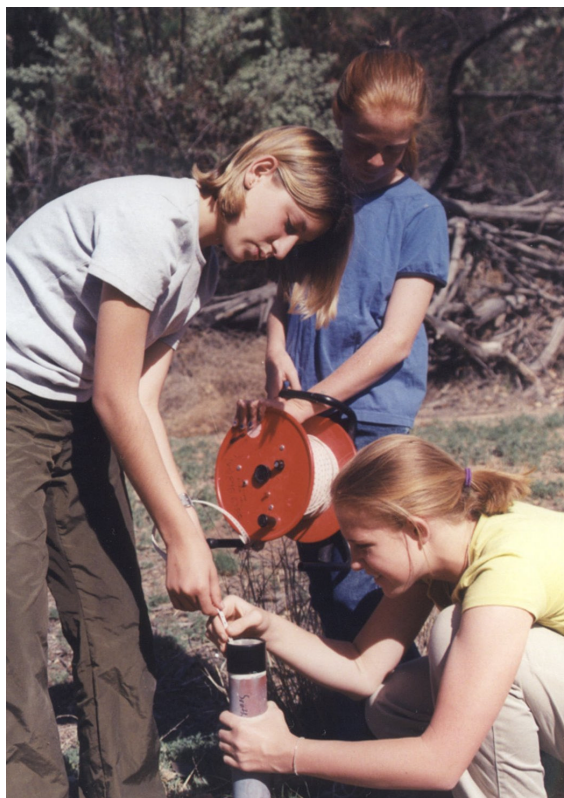
Later, students use a beeper or water level meter to measure groundwater depth.
