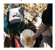
Data Collected Turbidity Dissolved Oxygen Temperature Conductivity pH and Lab Work: chloride, bromide, nitrate, phosphate, sulfate & ammonium
