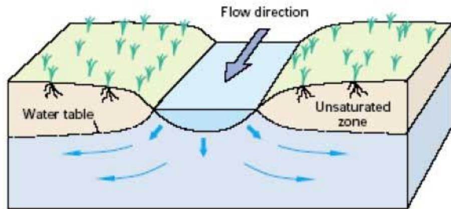
**Figure B-2: Gaining (Left) and Losing (Right) Streams and Associated Groundwater Flow Direction**
