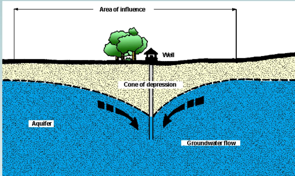
Pumping from a well in a water table aquifer **LOWERS** the water table near the well.
